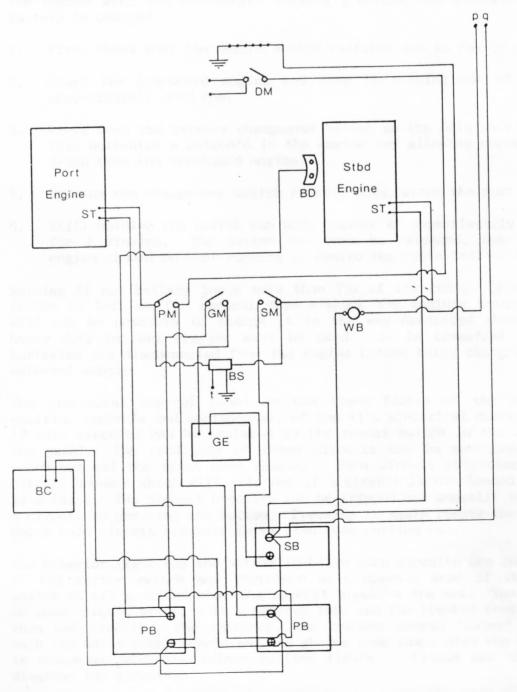
All master switches should be turned off when the boat is unattended and the winch should be isolated by pulling up the circuit breaker button. We also recommend that the engine master switches are turned off when the engines are not in use for any length of time. Never turn off the engine master switches when the engines are running as this will seriously damage the alternators.
