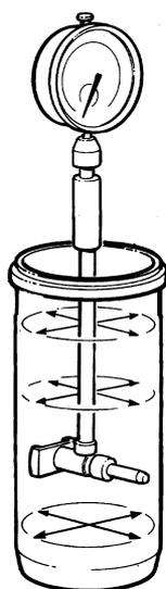
Measure the upper and lower turning points in the cylinder liner, and at several points along the height of the liner. At each measurement point, the measurement must be done in the transverse and lengthwise directions of the engine.
